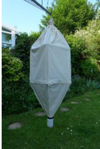
Example of a Winkler Extractor
