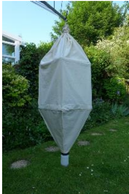
Example of a Winkler Extractor
