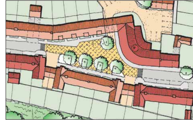
The formation of well designed squares can cater for on-street parking as well as providing interest within the street - scene
